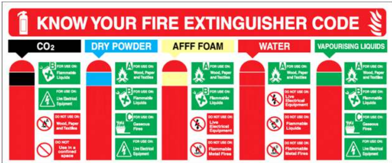
Fig 8.4.1.2 Know your fire extinguisher code
