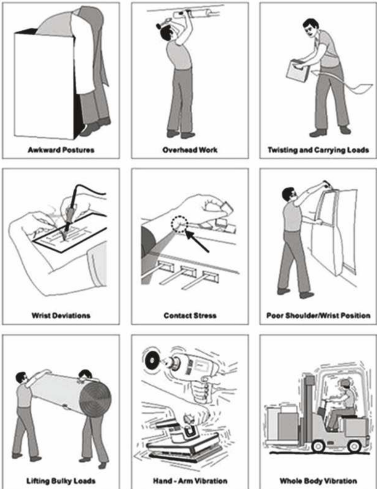
Fig 8.3.1.4 Problems to avoid
