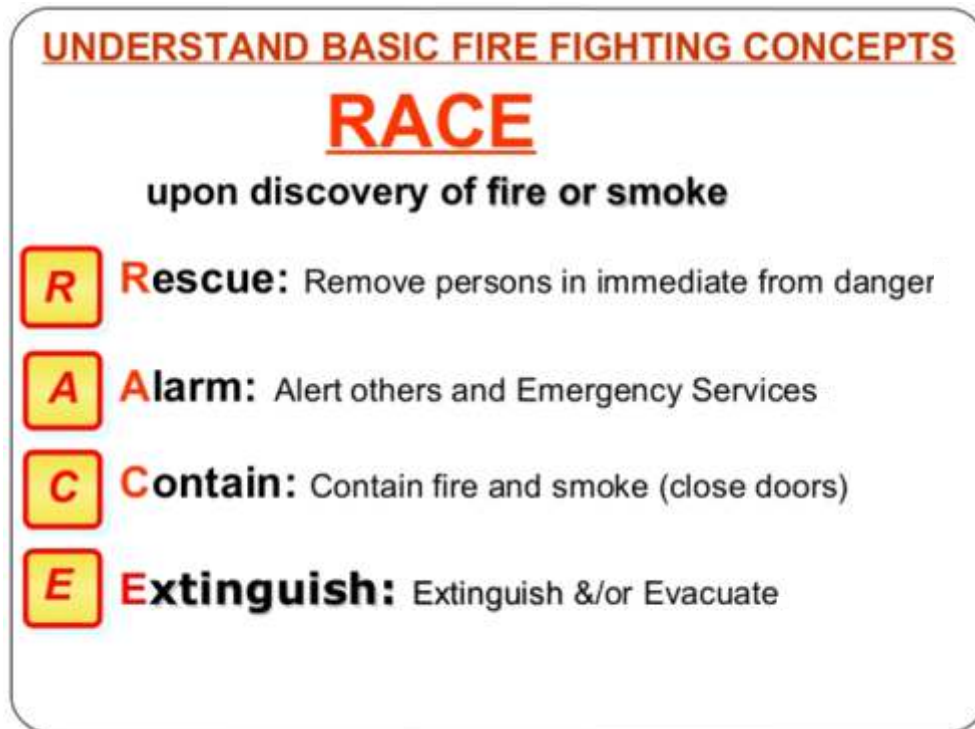
Fig 8.4.1.4 Basic fire fighting steps
